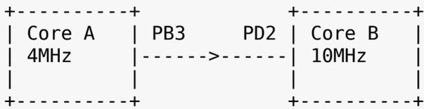
Core A runs as a 250Hz clock generator on pin B3. B3 from core A is connected with pin D2 on core B. Core B counts now all rising edges on pin D2 and measures the time distance between 2 events with timer T0.
