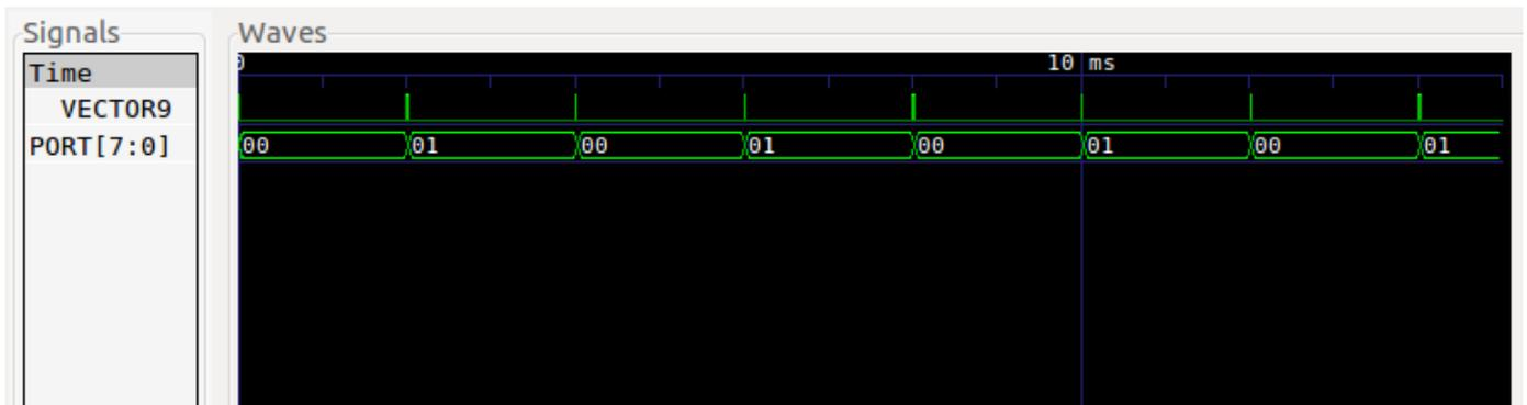
Let's look on a detail. You can see, how long the interrupt procedure was running and when the port value was changed. Compare it with the print out on standard out before! (in picture the value for "Marker:")
