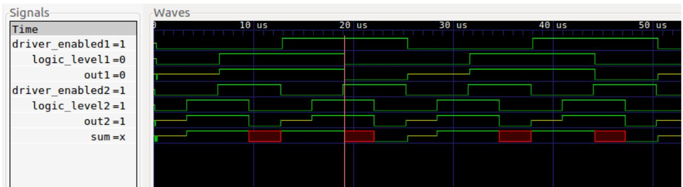
driver\_enabledX (X is 1 or 2 for core 1 or core 2) shows the pin from the port driven by coreX - this represents DDR bit. logic\_levelX represents the setting of PORT bit. outX represents the resulting signal from above values.
