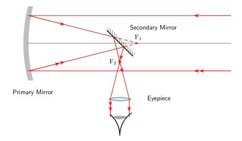
Figure 13.21: Lenses and mirrors in a reflecting telescope.
