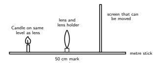
Figure 13.6: Experimental setup for investigation.
