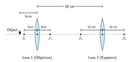
Step 2: Find the image for the objective lens.
