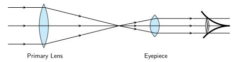
Figure 13.20: Layout of lenses in a refracting telescope
