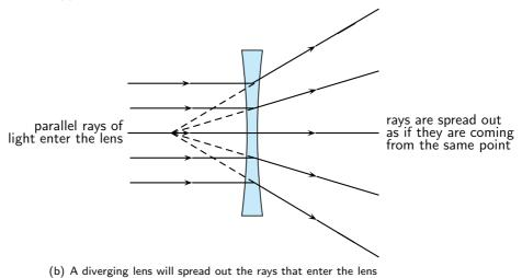
Figure 13.1: The behaviour of parallel light rays entering either a converging or diverging lens.
